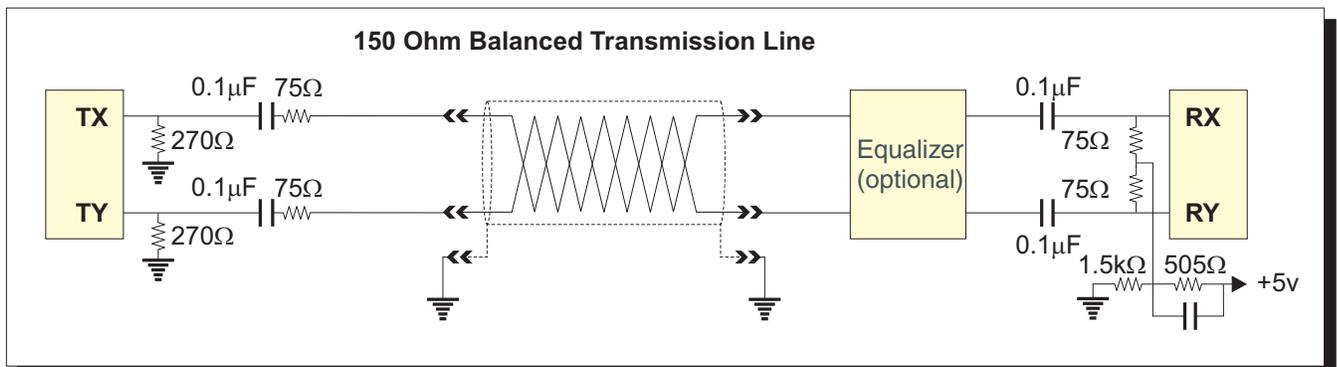
**Figure 34. Differential Transmit and Receive Networks**
