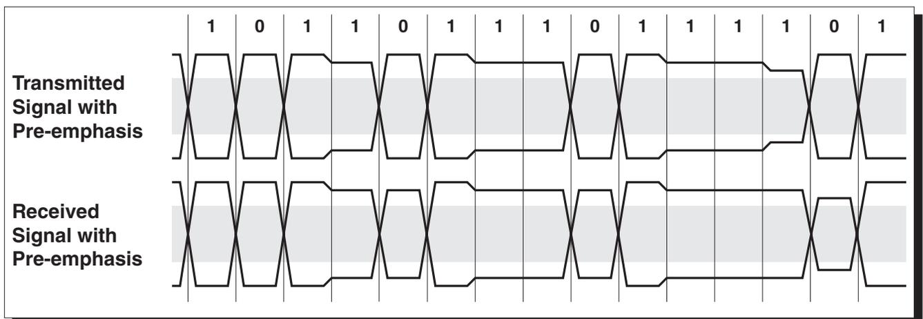
**Figure 38. Transmit Signal With De-Emphasis**
