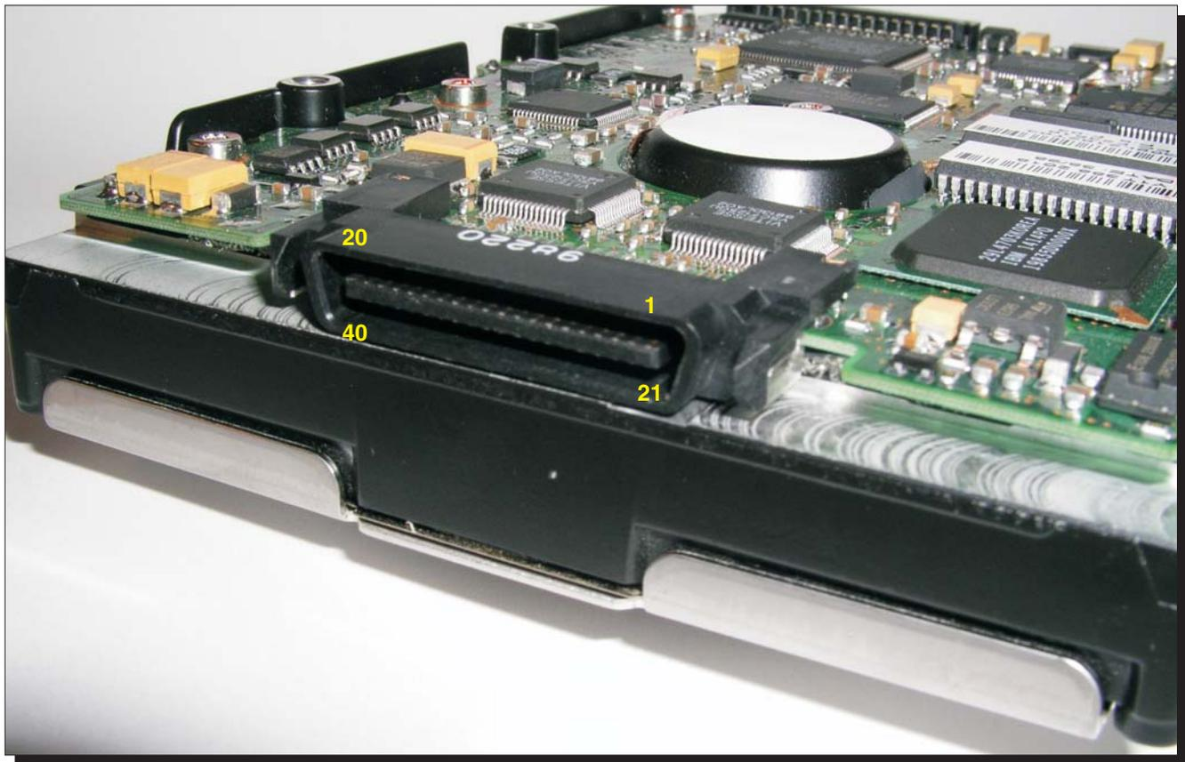
**Figure 44. SCA-2 40-Pin Disk Connector**
