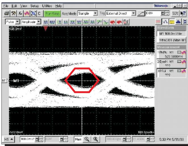
Figure 36. Eye Diagram (10 Meter Cable)
