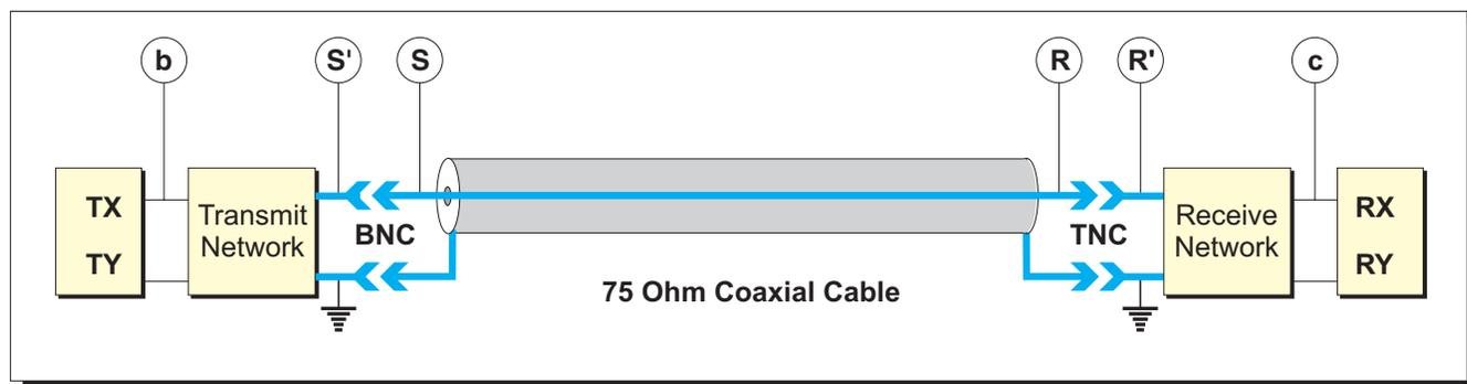
**Figure 31. Single-Ended, Unbalanced Link**
