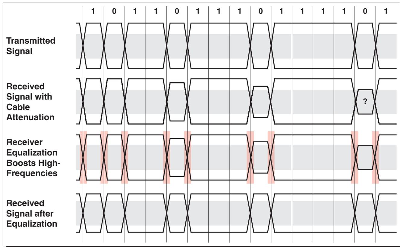
**Figure 41. Receiver Equalization**
