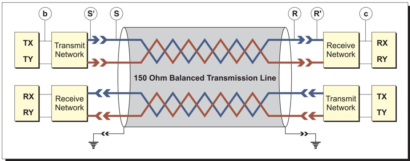
**Figure 32. Differential, Balanced Link**
