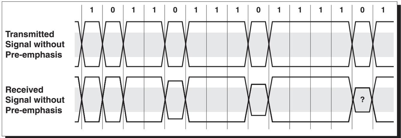
**Figure 37. Transmit Signal Without De-Emphasis**
