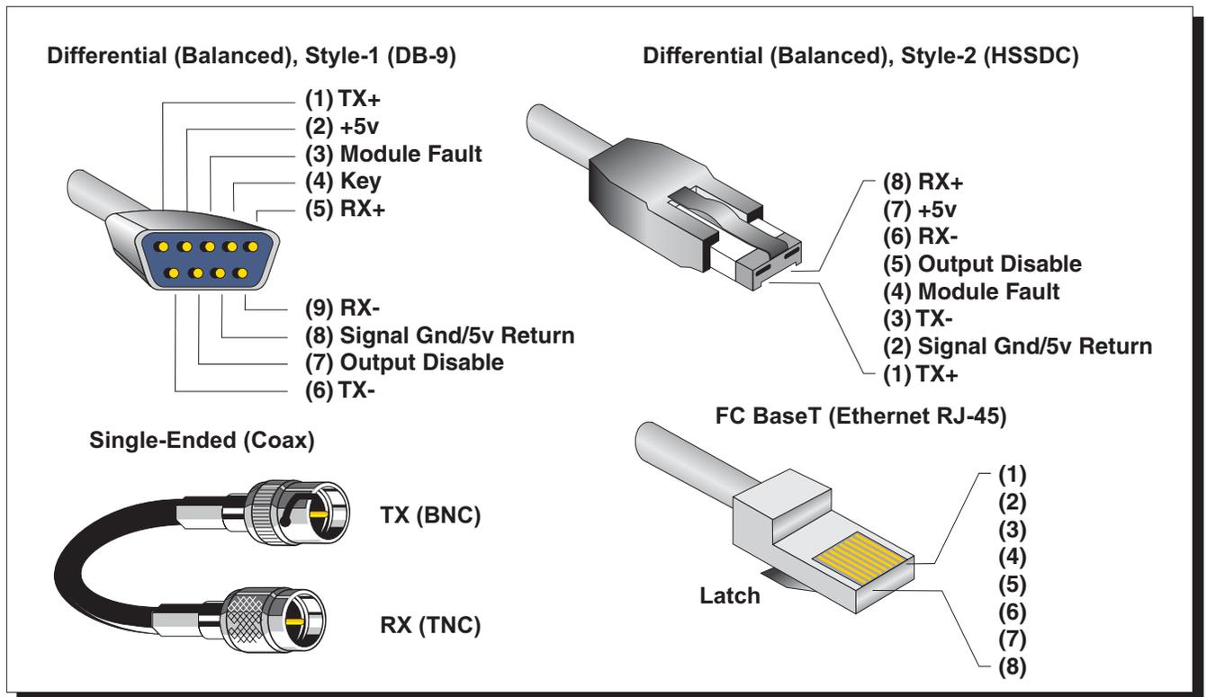
**Figure 43. Connectors for Electrical Interfaces**
