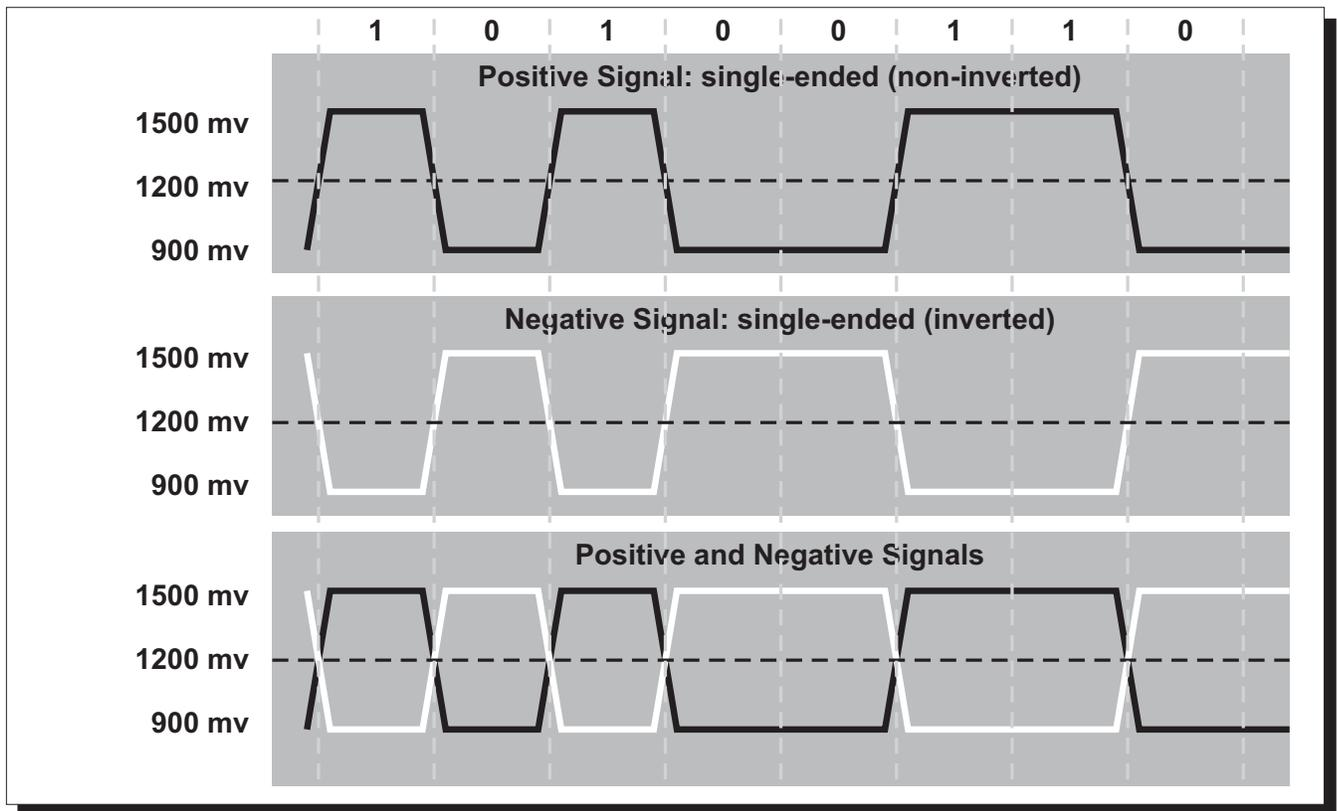
**Figure 33. Differential Signaling Example**
